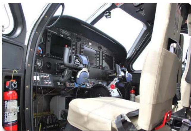
The Kodiak cockpit features the latest satellite navigation in its "all glass" instrument panel.
